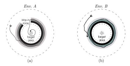
Figure 4: Depiction of the task. (a) *Env. A* is characterised by the way in zone. The target area, centred on the light, is indicated by the dashed circle. (b) In *Env. B* there is no way in zone and the target area cannot be reached. The continuous lines are an example of a good navigation strategy for one robot.
