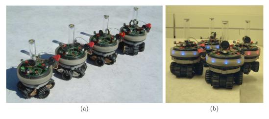
Figure 2: (a) Four real s-bots forming a linear swarm-bot during coordinated motion. (b) A physical swarm-bot while performing hole avoidance. Notice how physical connections among the s-bots can serve as support when a robot is suspended out of the arena, still allowing the whole system to work.
